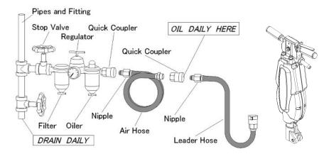
Whether there is any dust, or damage to the air connection portion. Whether the air hose is tight enough.
